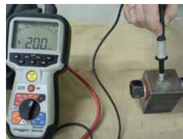
HC washer with ZP steel back-up washer bolted to washer test block. Megger isolation test unit confirms full 200G Ohm isolation at 1000V.
